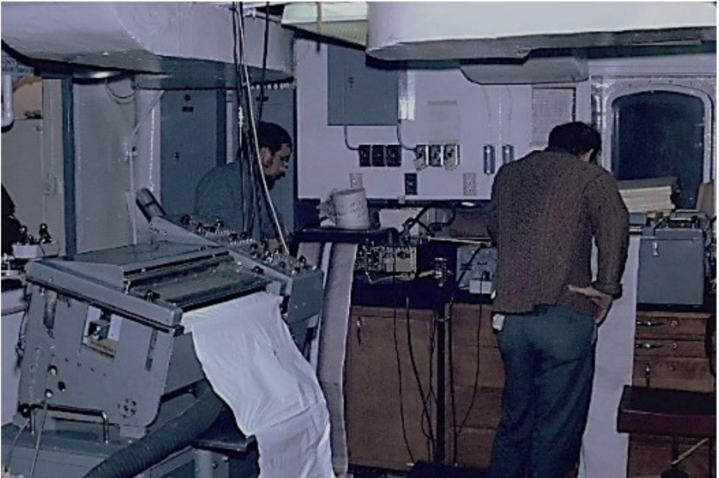
Figure 1 Operations laboratory onboard CSS Hudson , 1970. Left: Continuous seismic reflection profile of the sub-seabed generated by Hunttec 2A recorder. Centre: Peter Wadhams, graduate student participant, observing seabed saturated by ice scours on a continuous sidescan sonar profile generated by EGG Mark 1 recorder. Right: Jim Shearer observing seabed topography of a pingo-like feature on continuous bathymetric profile on a Raytheon recorder. Photo Credit: Roger W. Smith, student participant, Hudson 70 .
