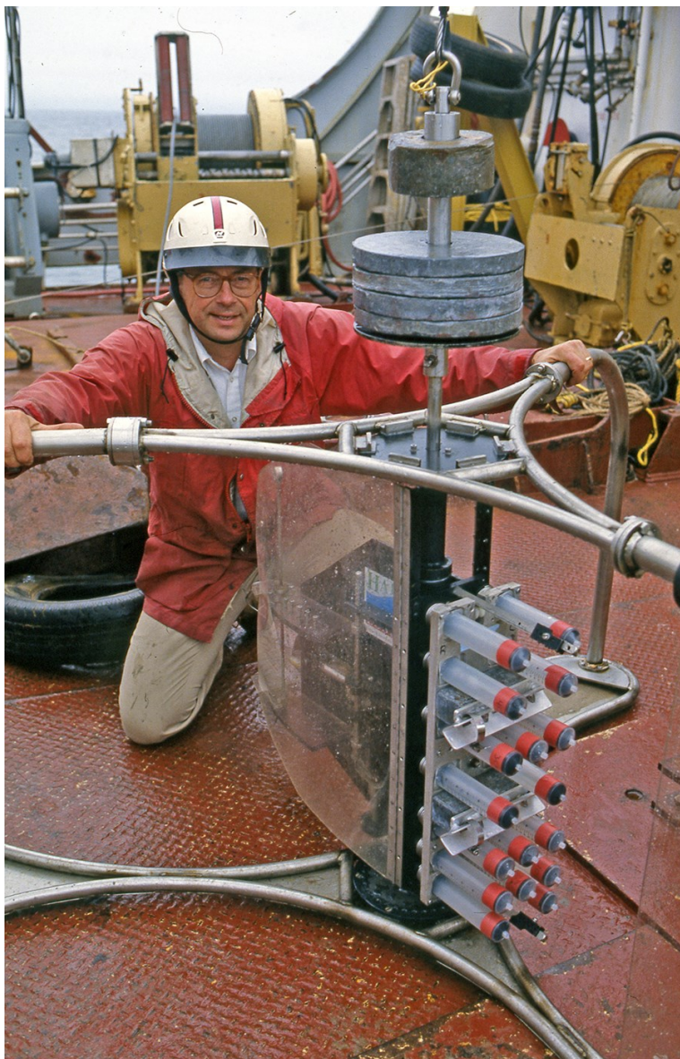
Don Gordon preparing the BOSS (Benthic Organic Seston Sampler) for deployment on the deck of CSS Parizeau in the mid-1990's Photo credit: BIO Photo Unit
