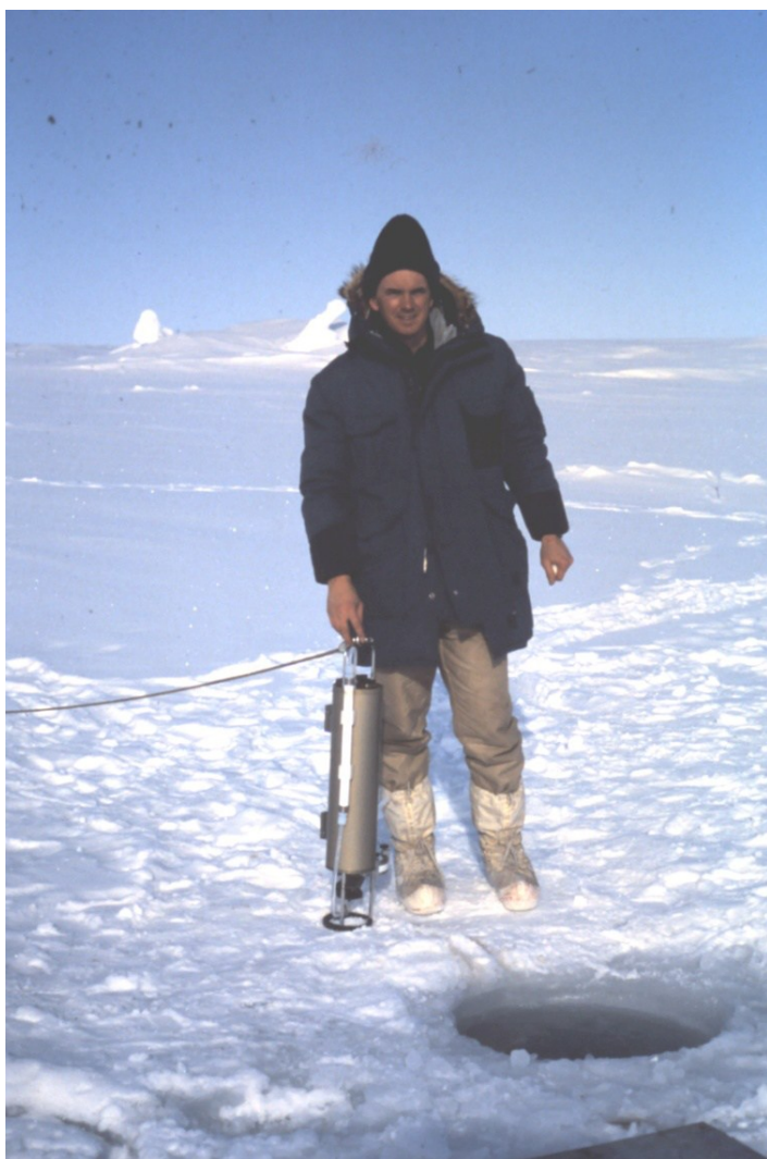
Barry Hargrave with a Seastar pump used to extract OCs from seawater.
